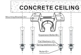
Note: According to the ceiling of different materials, use different screws to fix the hanging bracket. Don't fix the hanging bracket on the wood ceiling less than 12MM to prevent danger caused by
