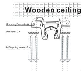
For wooden ceiling, use wood screw to drill on the wooden beam or the "junction box" to fix the hanging bracket (selection is made according to actual requirements of the customers).
